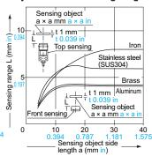
As the sensing object size becomes smaller than the standard size (iron sheet  $30 \times 30 \times 11 \text{ mm } 1.181 \times 1.181 \times 10.039 \text{ in}$ ), the sensing range shortens as shown in the left figure.
