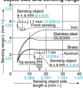
As the sensing object size becomes smaller than the standard size (iron sheet  $20 \times 20 \times t$  1 mm  $0.787 \times 0.787 \times t$  0.039 in), the sensing range shortens as shown in the left figure.
