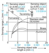
As the sensing object size becomes smaller than the standard size (iron sheet  $15 \times 15 \times t\ 1\ \text{mm}\ 0.591 \times 0.591 \times t\ 0.039$  in), the sensing range shortens as shown in the left figures.
