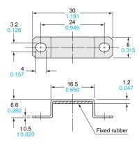
Material: Bracket ... Stainless steel (SUS304) Fixed rubber ... FKM (Fluorine rubber) MS-GXL15 Sensor mounting bracket for GXL-15 type (Optional)
