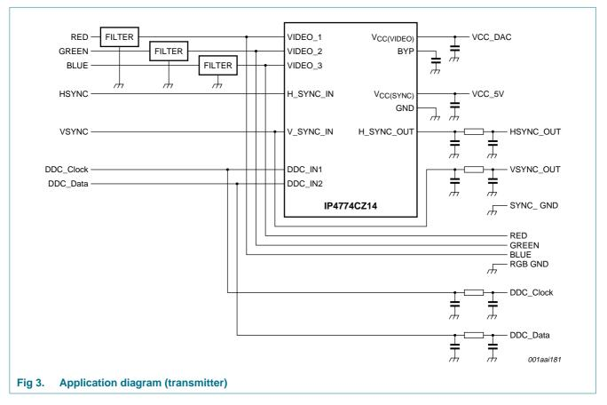
The IP4774CZ14 is connected to the input lines of the VGA connector to protect the VGA port including all signals and buffering of the h-sync signal.
