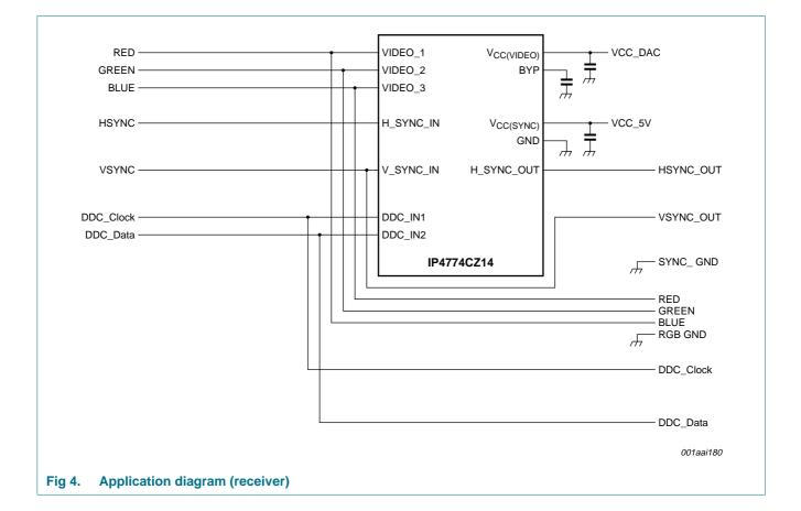
VGA port protection with sync buffer
