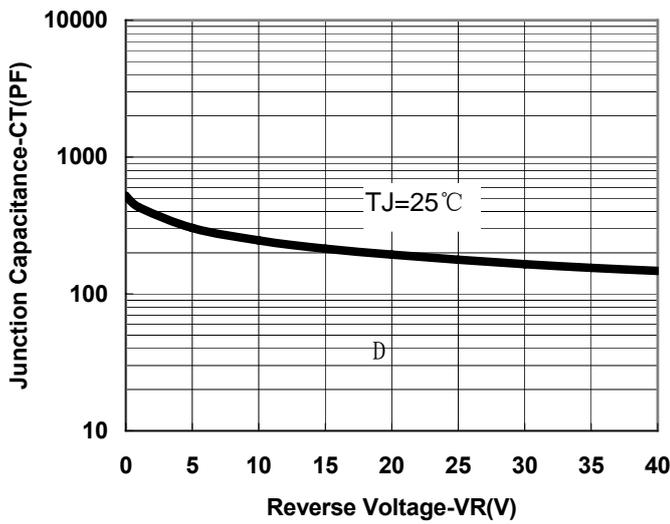
Fig.1-Typical Junction Capacitance
