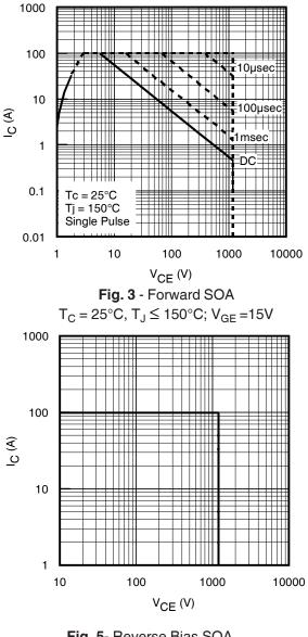
Fig. 5- Reverse Bias SOA  $T_J = 150^{\circ}$ C;  $V_{GE} = 20V$
