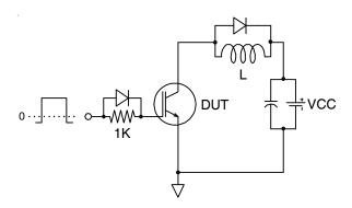
Fig.C.T.1 - Gate Charge Circuit (turn-off)
