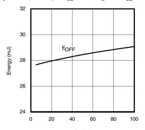
Rg (Ω) Fig. 15 - Typ. Energy Loss vs. R<sub>G</sub>  $T_J = 150^{\circ}C$ ; L = 400µH; V<sub>CE</sub> = 600V, I<sub>CE</sub> = 33A; V<sub>GE</sub> = 15V
