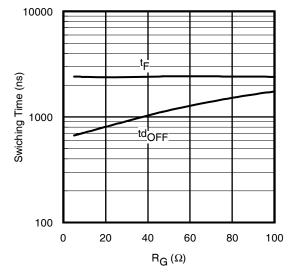
Fig. 16- Typ. Switching Time vs. R<sub>G</sub>  $T_J = 150^{\circ}C; L = 400 \mu H; V_{CE} = 600V, I_{CE} = 33A; V_{GE} = 15V$
