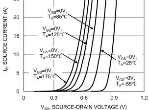
Figure 9. Diode Forward Voltage vs. Current
