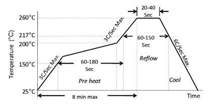
Figure 3. Solder Reflow Profile
