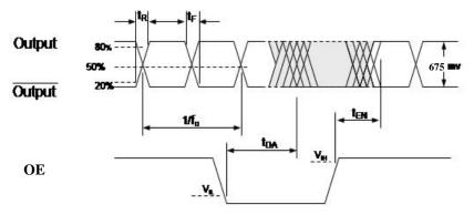
Figure 2. HCSL Output Waveform
