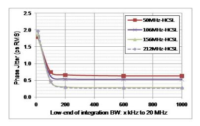
Figure 1. HCSL Phase Jitter (integrated phase noise)
