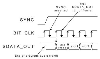
SDATA\_OUT's composite stream is MSB justified (MSB first) with all non-valid slots' bit positions stuffed with 0 by the AC'97 Controller. If there are less than 20 valid bits within an assigned and valid time slot, the AC'97 Controller always stuffs all trailing non-valid bit positions of the 20-bit slot with 0.
