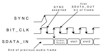
SDATA\_IN's composite stream is MSB justified (MSB first) with all non-valid bit positions (for assigned and/or unassigned time slots) stuffed with 0 by the AC'97 CODEC. SDATA\_IN data is sampled on the falling edges of BIT\_CLK.
