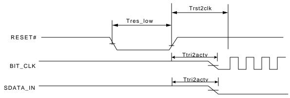
Figure 1. Cold Reset Timing
