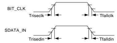
Figure 5. Signal Rise and Fall Times Timing
