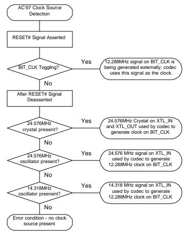
Figure 11. CODEC Clock Source Detection
