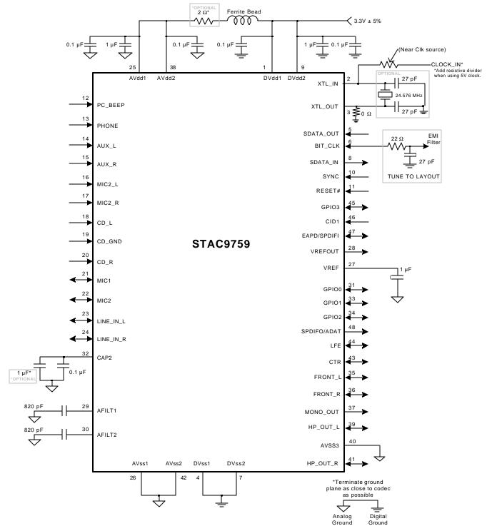
Figure 9. Split Independent Power Supply Operation
