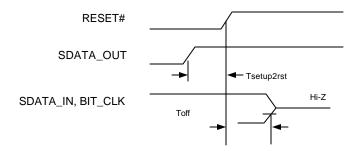
Figure 7. ATE Test Mode Timing
