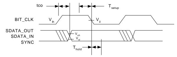
Figure 4. Data Setup and Hold Timing
