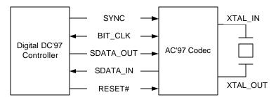
Figure 10. AC-Link to its Companion Controller
