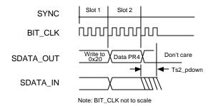
Figure 6. AC-Link Low Power Mode Timing
