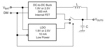
Low undershoot voltage is expected when going from PWM to LDO mode and viceversa. The circuit is designed in order to avoid any spikes when transition between two modes is enabled.
