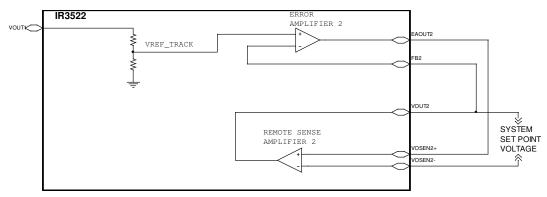
Figure 2B - Output 2 System Set Point Test Circuit
