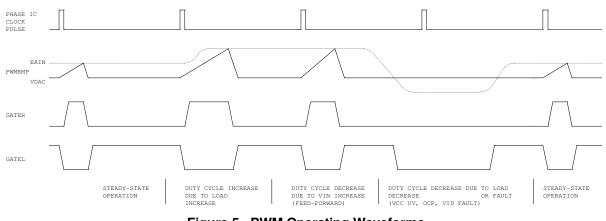
Figure 5 PWM Operating Waveforms
