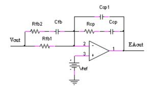
Figure 12 Voltage Loop Compensation Network
