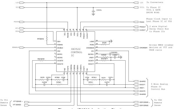
Figure 1 – IR3522 Application Circuit
