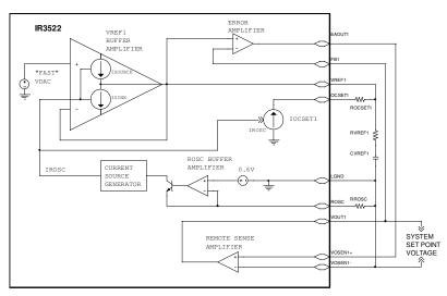
Figure 2A - Output 1 System Set Point Test Circuit
