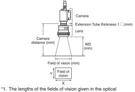
The lengths of the fields of vision given in the optical charts are the lengths of the Y axis.
