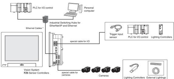
\* To use Straight or cross STP (shielded twisted-pair) cable of category 5 or higher for Ethernet and RJ45 connector.
