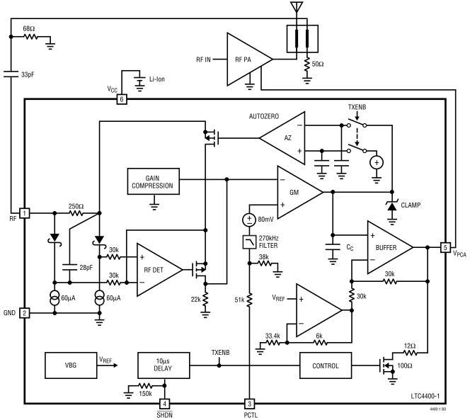
NOTE: THE DIRECTIONAL COUPLER SHOWN IN THIS FIGURE MAY BE REPLACED WITH A COUPLING CAPACITOR AND RESISTOR AS DESCRIBED IN APPLICATION NOTE 91 "LOW COST COUPLING METHODS FOR RF POWER DETECTORS REPLACE DIRECTIONAL COUPLERS"
