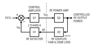
Figure 4. Closed-Loop Block Diagram
