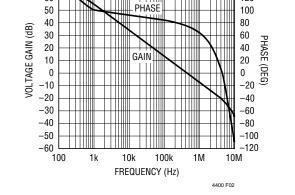
Figure 2. Measured Open-Loop Gain and Phase, PCTL < 80mV
