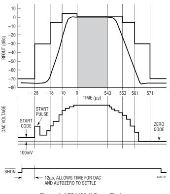
Figure 1. LTC4400-X Ramp Timing
