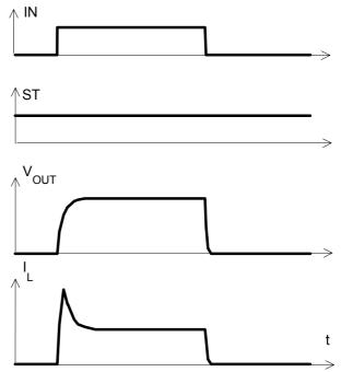
The initial peak current should be limited by the lamp and not by the current limit of the device.
