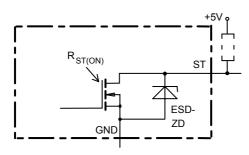
ESD-Zener diode: 6.1 V typ., max 5.0 mA;  $R_{ST(ON)}$  < 375  $\Omega$  at 1.6 mA. The use of ESD zener diodes as voltage clamp at DC conditions is not recommended.
