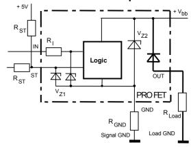
$V_{Z1}$  = 6.1 V typ.,  $V_{Z2}$  = 47 V typ.,  $R_{GND}$  = 150 Ω,  $R_{ST}$ = 15 kΩ,  $R_{I}$ = 3.5 kΩ typ.
