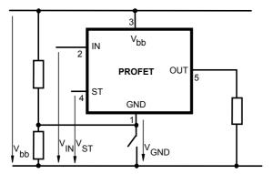
Any kind of load. If  $V_{GND}$  >  $V_{IN}$  -  $V_{IN(T+)}$  device stays off Due to  $V_{GND}$  >0, no  $V_{ST}$  = low signal available.
