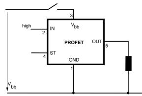
For inductive load currents up to the limits defined by Z<sub>L</sub> (max. ratings and diagram on page 8) each switch is protected against loss of V<sub>bb</sub>.
