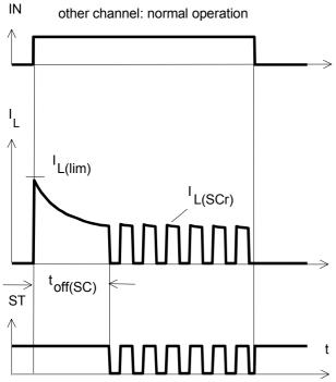
Heating up of the chip may require several milliseconds, depending on external conditions
