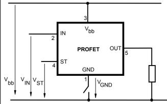
Any kind of load. In case of Input=high is  $V_{OUT} \approx V_{IN} - V_{IN(T+)}$ . Due to  $V_{GND}$  >0, no  $V_{ST}$  = low signal available.
