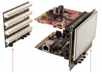
Please attach a primary TWR-ELEV module along with MCU and peripheral modules for complete Tower System assembly.
