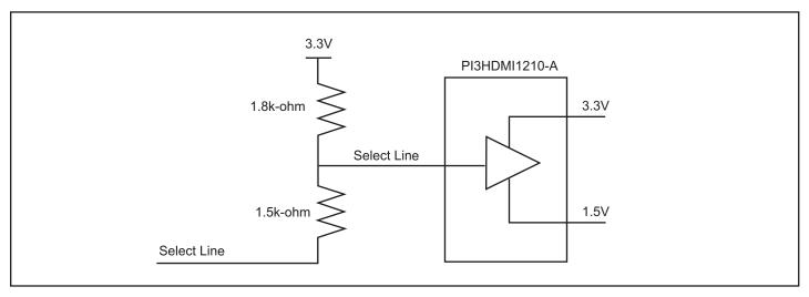
Example of a circuit that needs to be connected to the SEL pin (8) of the PI3HDMI1210-A of our device
