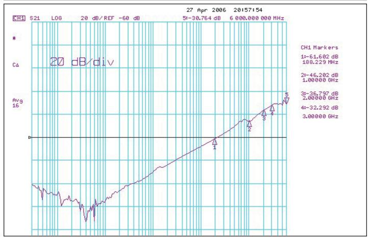
Fig 3. Crosstalk for High-speed data signals only
