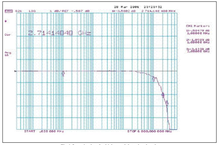
Fig 4. Insertion loss for high-speed data signals only
