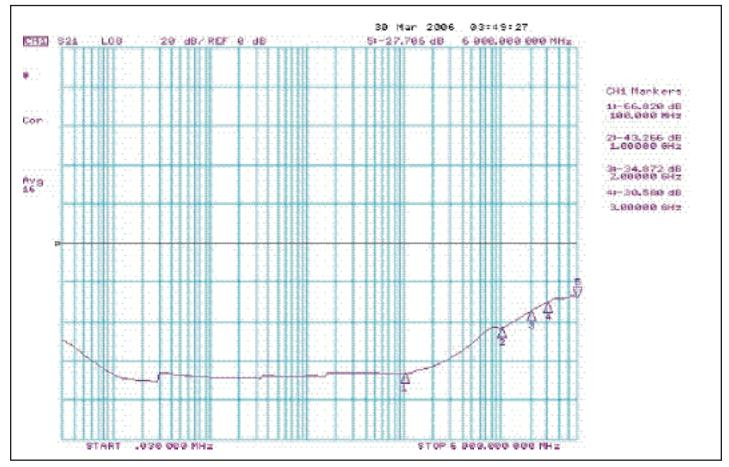
Fig 4. Off Isolation for high-speed data signals only
