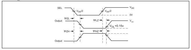
**Voltage Waveforms Enable and Disable Times**
