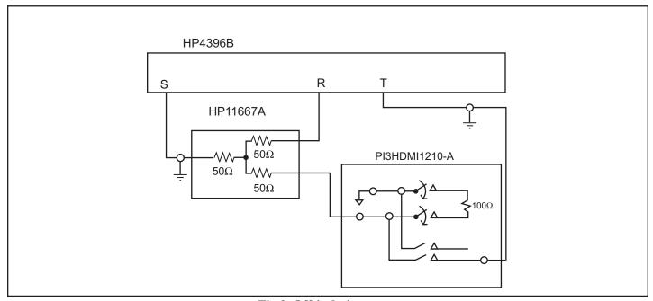
Fig 2. Off-isolation setup
