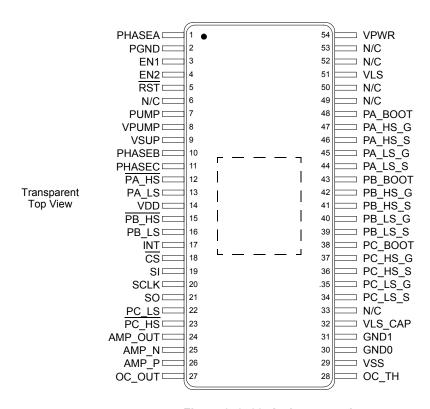
Figure 3. 34937A pin connections
