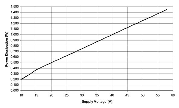
Figure 25. Power dissipation profile of application not using charge pump
