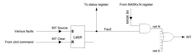
Figure 18. Interrupt handling
