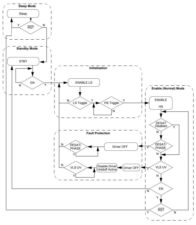
Figure 17. Device operational flow diagram
