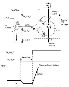
Figure 14. Positive dv/dt transient
