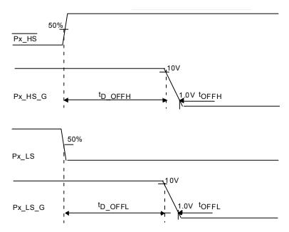
Figure 8. Driver turn-off time and turn-off delay
