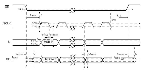
Figure 4. SPI interface timing
