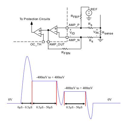
Figure 9. Current amplifier and input waveform ( $V_{\text{IN}}$  voltage across  $R_{\text{SENSE}}$ )
