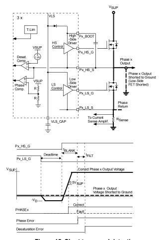
Figure 15. Short to ground detection
