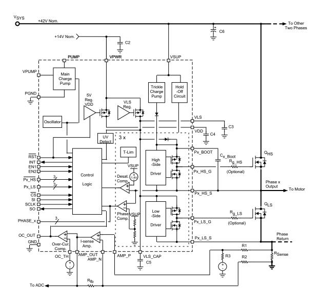
Figure 23. High-voltage application diagram (+42 V system)
