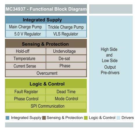
Figure 12. Functional internal block description
