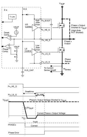
Figure 16. Short to supply detection
