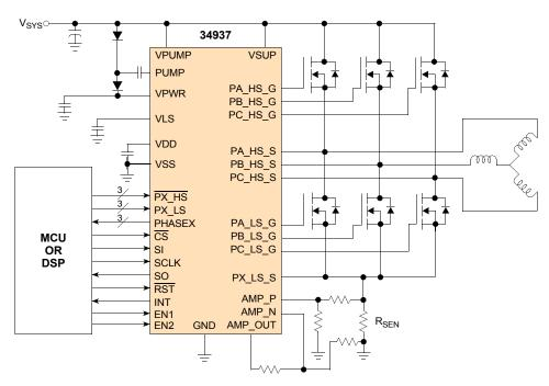
Figure 1. 34937A simplified application diagram
