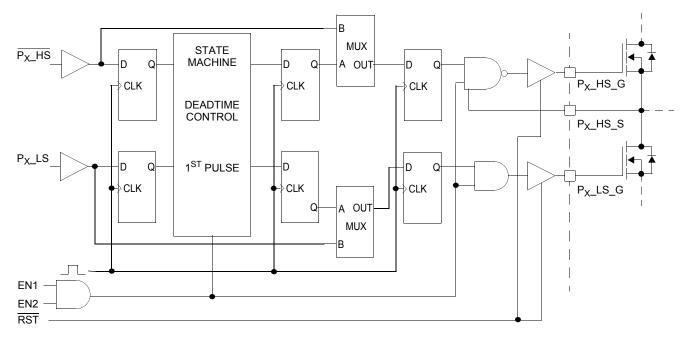
Figure 6. Deadtime control delays
