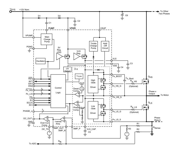
Figure 22. Typical application diagram using charge pump
