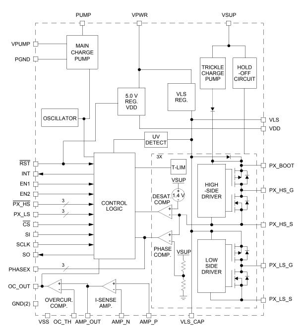
Figure 2. 34937A simplified internal block diagram
