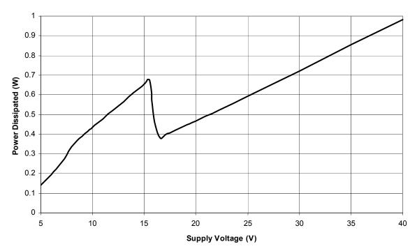
Figure 24. Power dissipation profile of application using charge pump
