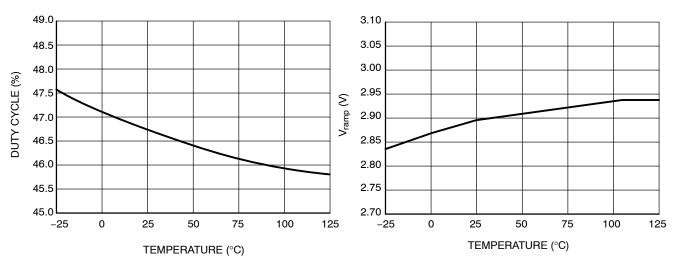
Figure 15. NCP1216A Max Duty-Cycle vs. Temperature
