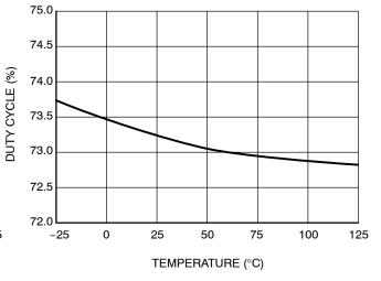
Figure 13. V<sub>skip</sub> vs. Temperature
