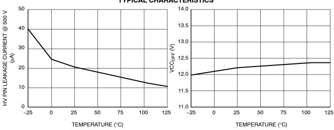
Figure 3. High Voltage Pin Leakage Current vs. Temperature
