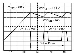
Figure 18. The Charge/Discharge Cycle Over a 10 μF V<sub>CC</sub> Capacitor
