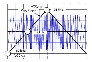
Figure 20. V<sub>CC</sub> Ripple is Used to Introduce a Frequency Jittering on the Internal Oscillator Sawtooth
