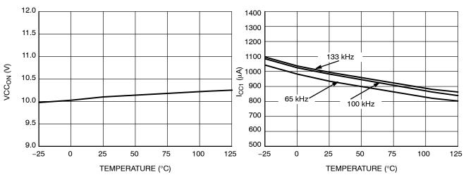
Figure 5. VCC<sub>ON</sub> vs. Temperature
