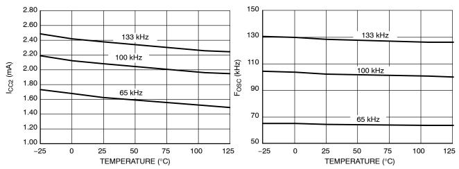
Figure 7. I<sub>CC2</sub> vs. Temperature
