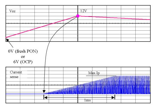
Figure 29. Soft-start is activated during a startup sequence or an OCP condition
