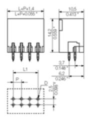
1728860000 S2L 3.5/20/180G3.5SN OR PCB plug-in connector, Male connectors, Soldered connection, Pitch: 3.50 mm, No. of poles: 20, 180°, Box 4032248036899 20 pc(s).
