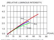
FIG.2 RELATIVE LUMINOUS INTENSITY VS. FORWARD CURRENT
