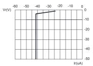
FIG.3a RED REVERSE CURRENT VS. REVERSE VOLTAGE.
