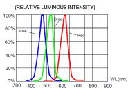
FIG.5 RELATIVE LUMINOUS INTENSITY VS. WAVELENGTH.
