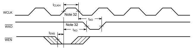
Figure 17. Read Expansion Out Timing
