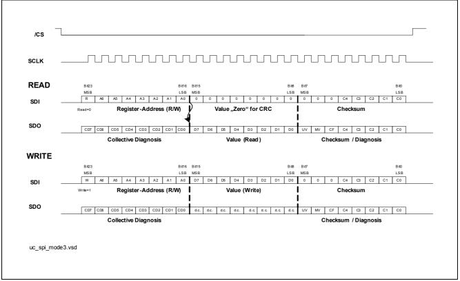
Figure 15 SPI Mode 3, MS0 = 1, MS1 = 1
