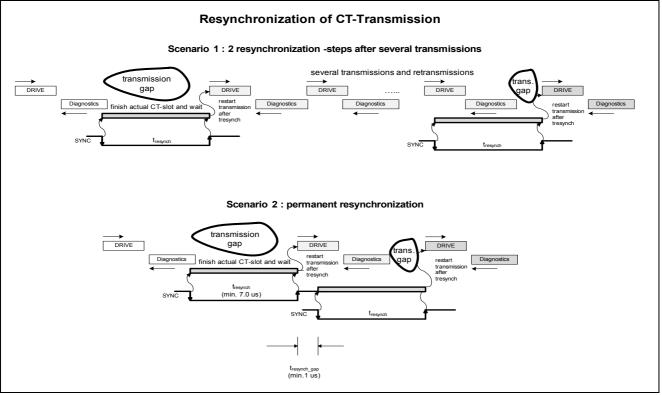
Figure 20 Examples of Application of Resynchronization
