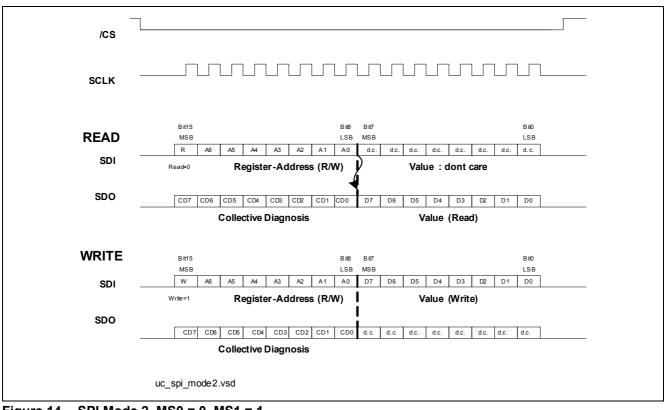
Figure 14 SPI Mode 2, MS0 = 0, MS1 = 1
