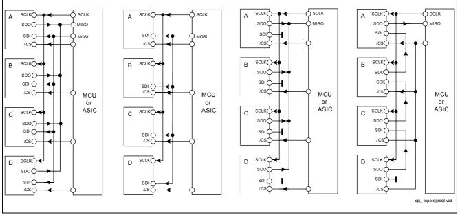
Figure 11 Example SPI Topologies
