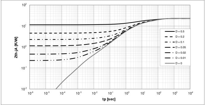
Figure 36 Typ. Transient Thermal Impedance 2s2p
