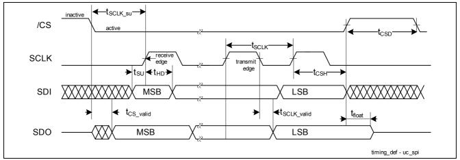
Figure 10 Serial Bus Timing
