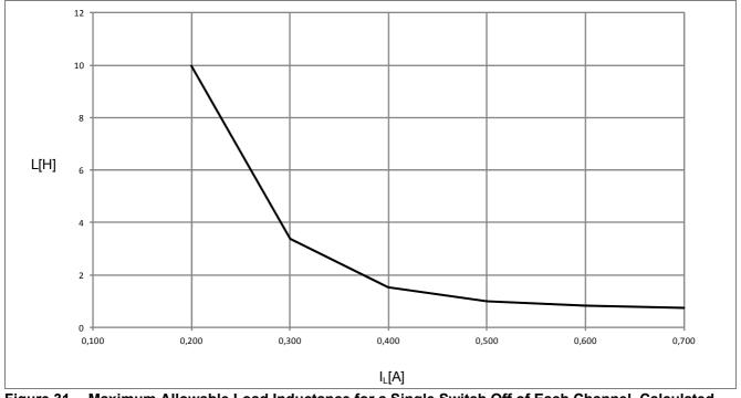
**Figure 31** Maximum Allowable Load Inductance for a Single Switch Off of Each Channel, Calculated  $L = f(I_L)$ ,  $T_{jstart} = 125$  °C,  $V_{BB} = 24$  V,  $R_L = 48 \Omega$ , all channels are switching simultaneously
