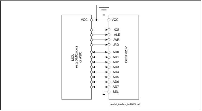
Figure 6 Bus Configuration for Parallel Mode
