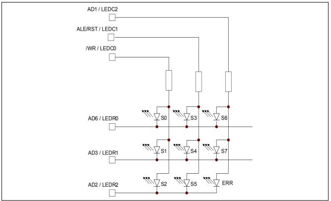
Figure 25 LED Matrix connected to the uC-Chip
