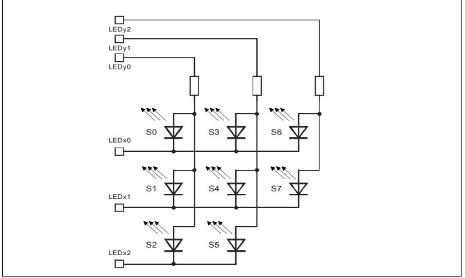
Figure 23 LED Matrix connected to the Power Chip
