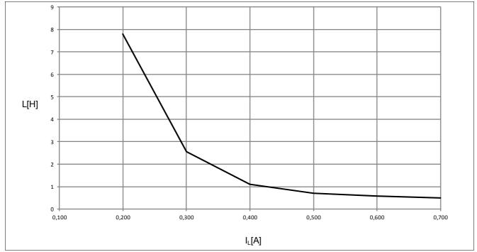
**Figure 32** Maximum Allowable Load Inductance for a Single Switch Off of Each Channel, Calculated  $L = f(I_L)$ ,  $T_{istart} = 125 \text{ °C}$ ,  $V_{BB} = 24 \text{ V}$ ,  $R_L = 0 \Omega$ , all channels are switching simultaneously
