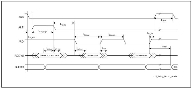
The timing requirements for the parallel interface are shown in Figure 7 (Read), Figure 8 (Write) and Table 23.
