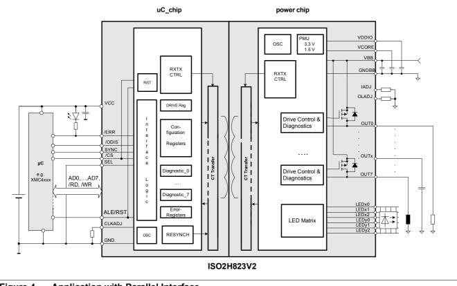
Figure 4 **Application with Parallel Interface**
