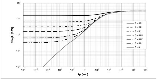
Figure 35 Typ. Transient Thermal Impedance 2s2p no vias
