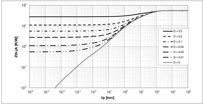
Figure 34 Typ. Transient Thermal Impedance 1s0p
