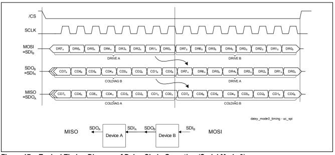
Figure 17 Typical Timing Diagram of Daisy Chain Operation (Serial Mode 0)
