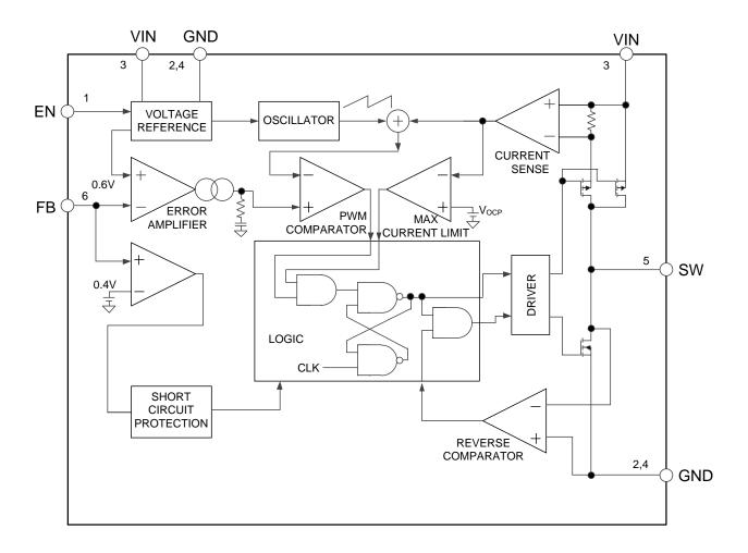
Figure 3 · Simplified Block Diagram of LX7188
