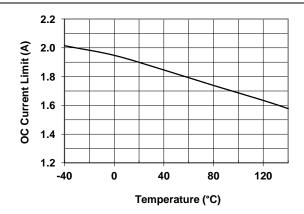
Figure 10 · OCP Current Limit vs. Temperature
