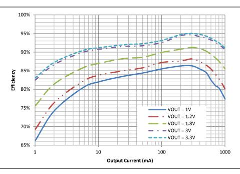
Figure  $4 \cdot \text{Efficiency vs. Output Current with 5V Input}$
