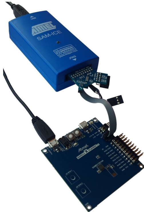
Figure 5-7. SAM-ICE using an Atmel-ICE Adapter
