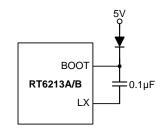
Figure 6. External Bootstrap Diode
