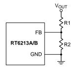
Figure 5. Output Voltage Setting
