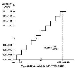
Figure 15. AD7858/AD7858L Transfer Characteristic
