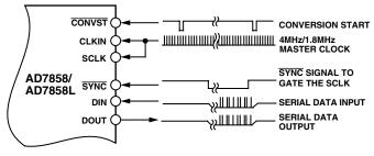
Figure 36. Simplified Interface Diagram
