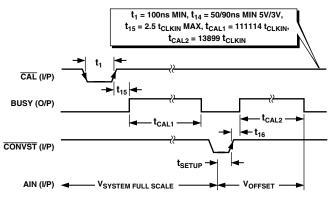
Figure 29. Timing Diagram for Full System Calibration
