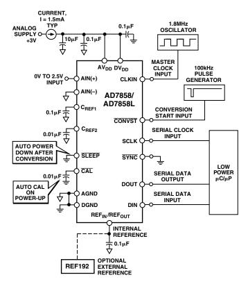
Figure 21. Typical Low Power Circuit
