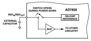
Figure 23. On-Chip Reference During Power-Down
