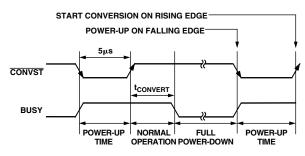
Figure 22. Power-Up Timing When Using CONVST Pin
