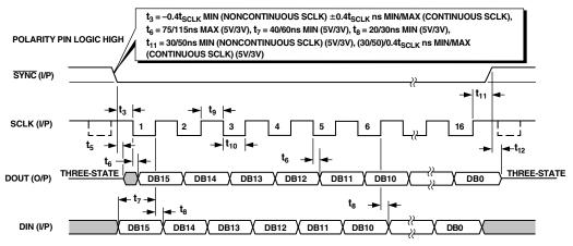
Figure 33. SPI/QSPI Mode 2 Timing Diagram for Read/Write Operation with DIN Input, DOUT Output, and SYNC Input
