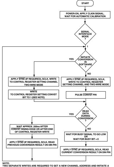
TWO SEPARATE WRITES ARE REQUIRED TO SET A NEW CHANNEL ADDRESS AND INITIATE A CONVERSION ON THAT NEW CHANNEL IN SOFTWARE AS THE ACQUISITION TIME (2  $t_{CLKIN}$ ) MUST ELAPSE BEFORE THE CONVERSION BEGINS. IF BOTH COMMANDS ARE ISSUED IN THE ONE WRITE THE RESULT OF THIS CONVERSION SHOULD BE DISCARDED AND THE NEXT CONVERSION ON THAT SAME CHANNEL WILL PROVIDE CORRECT RESULTS.
