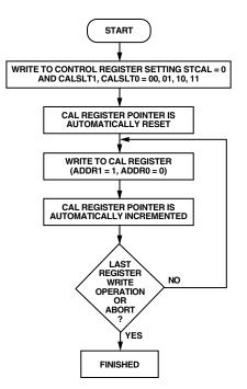
Figure 8. Flowchart for Writing to the Calibration Registers
