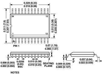
NOTES 1. LEAD NO. 1 IDENTIFIED BY A DOT. 2. LEADS WILL BE EITHER TIN PLATED OR SOLDER DIPPED IN ACCORDANCE WITH MIL-M-38510 REQUIREMENTS.
