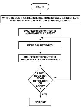
*Figure 9. Flowchart for Reading from the Calibration Registers*
