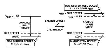
Figure 26. System Offset Calibration
