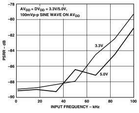
Figure 20. PSRR vs. Frequency
