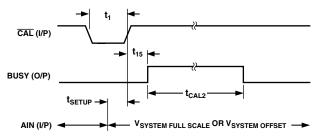
Figure 30. Timing Diagram for System Gain or System Offset Calibration
