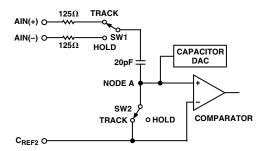
Figure 11. Analog Input Equivalent Circuit
