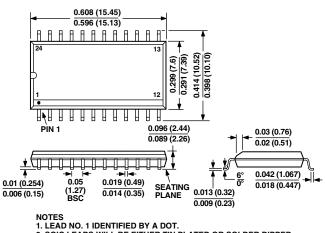
1. LEAD NO. 1 IDENTIFIED BY A DOT. 2. SOIC LEADS WILL BE EITHER TIN PLATED OR SOLDER DIPPED IN ACCORDANCE WITH MIL-M-38510 REQUIREMENTS.
