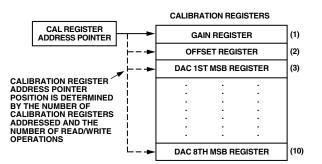
Figure 7. Calibration Register Arrangements
