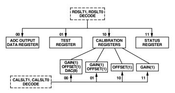
Figure 5. Read Register Hierarchy/Address Decoding
