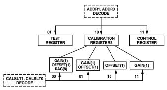
Figure 4. Write Register Hierarchy/Address Decoding
