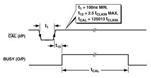
Figure 25. Timing Diagram for Full Self-Calibration
