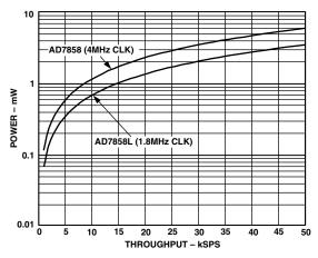
Figure 24. Power vs. Throughput Rate
