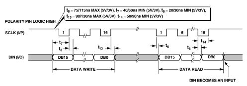
Figure 32. Timing Diagram for Read/Write Operation with DIN as an Input/Output and SYNC Input Tied Low (i.e., Interface Mode 1)
