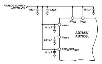
Figure 17. Relevant Connections When Using  $AV_{\text{DD}}$  as the Reference
