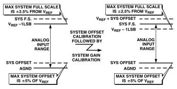
Figure 28. System (Gain + Offset) Calibration
