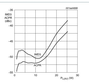
$V_{DS}$  = 28 V;  $I_{Dq}$  = 950 mA; f = 2140 MHz ( $\pm$  5 MHz); carrier spacing 10 MHz.
