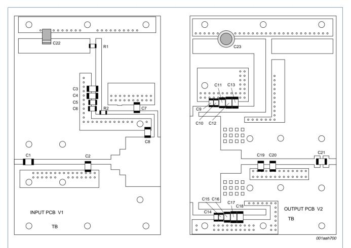
The striplines are on a double copper-clad Taconic RF35 Printed-Circuit Board (PCB) with  $\varepsilon_r$  = 3.5 and thickness = 0.76 mm. See Table 8 for list of components. The drawing is not to scale.
