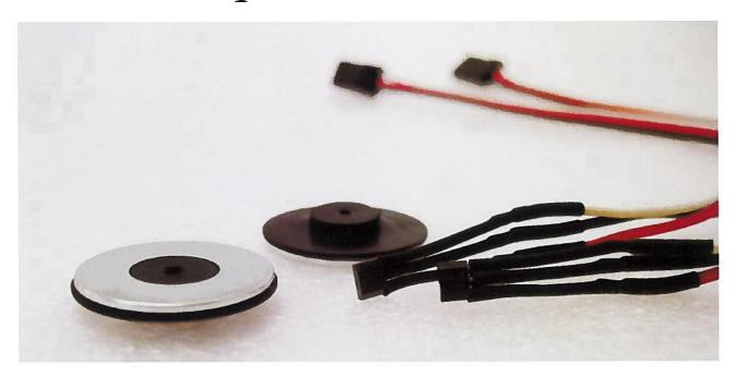
The simple encoder kit from DAGU consists of two neodymium 8-pole magnets with rubber hubs and two hall-effect sensors terminated with 150mm (6inch) cable and 3 pin female servo headers.
