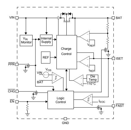
Figure 2. 34673 Simplified Internal Block Diagram
