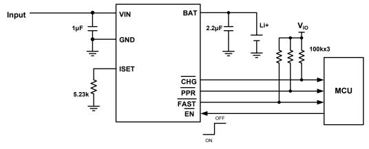
Figure 24. MCU Interfaced Charger
