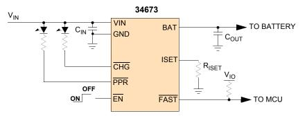
Figure 1. 34673 Simplified Application Diagram
