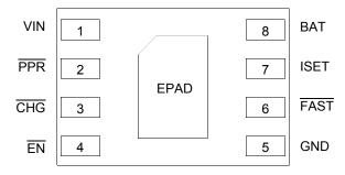
Figure 3. 34673 Pin Connections
