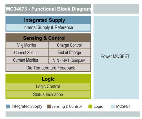
Figure 20. 34673 Functional Internal Block Diagram
