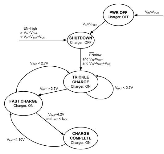
Figure 22. Charge Cycle State Diagram
