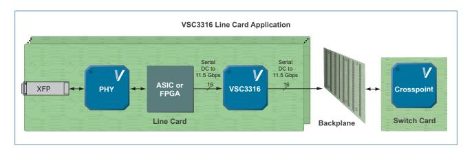
Using the VSC3316 in high-speed line cards ensures best-in-class I/O performance up to 11.5 Gbps with EQ technology to compensate for connector, backplane, and FR-4 loss.
