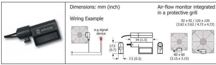
The air-flow monitor provides a simple alternative to indicate positive or negative air flow of fans or blowers. When properly installed and connected in series with an optical (i.e. LED) or audible signaling device, a bi-directional switch will activate an electrical contact if the air flow of the fan falls below 8.2 ft/s, turning the signaling device on or off. The AFM monitor can also be attached to an existing grill or guard.
