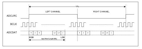
Figure 36 Left Justified Audio Interface (assuming n-bit word length)
