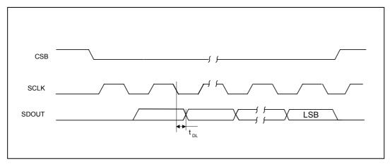
Figure 8 Control Interface Timing – 3-Wire Serial Control Mode (Read Cycle)
