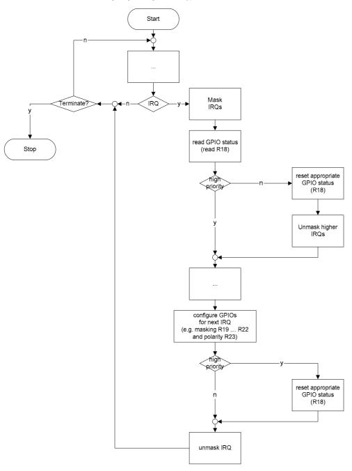
Figure 28 GPIO IRQ Handling
