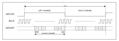
Figure 35 Right Justified Audio Interface (assuming n-bit word length)
