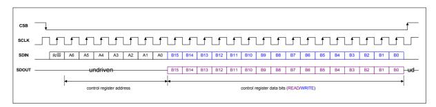
Figure 57 4-Wire Readback (wired-OR)
