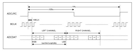
Figure 38 DSP Mode Audio Interface (mode A, AIF\_LRCLK\_INV=0, Master)
