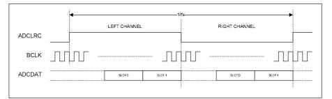
Figure 42 TDM in Right-Justified Mode
