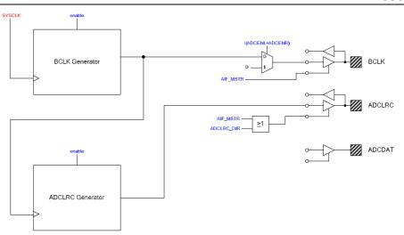
Figure 31 Audio Interface Output Control
