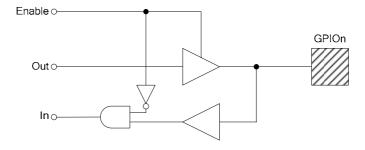
Figure 23 GPIO Pad
