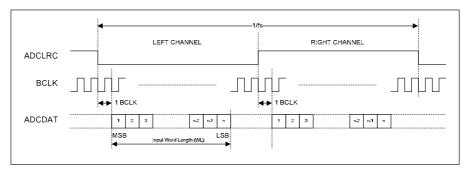
Figure 37 I2S Justified Audio Interface (assuming n-bit word length)
