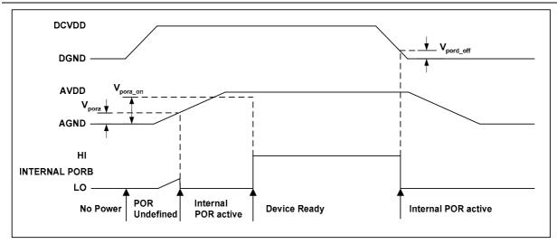
Figure 13 Typical Power up Sequence where DCVDD is Powered before AVDD
