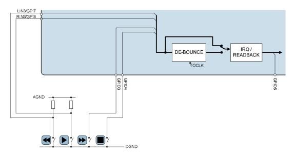
Figure 21 Example of Button Control Using GPIO Pins
