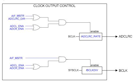
Figure 47 Clock Output Control
