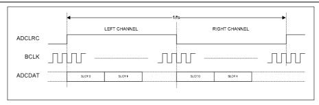
Figure 43 TDM in Left-Justified Mode
