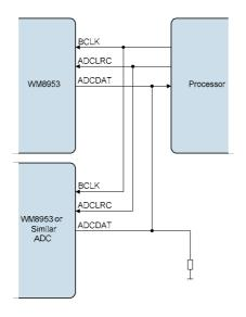
Figure 34 TDM with Processor as Master
