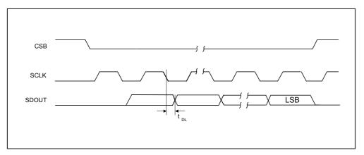
Figure 10 Control Interface Timing – 4-Wire Serial Control Mode (Read Cycle)
