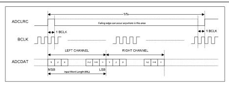
Figure 41 DSP Mode Audio Interface (mode B, AIF\_LRCLK\_INV=1, Slave)
