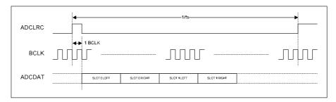
Figure 45 TDM in DSP Mode A
