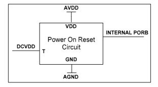
Figure 11 Internal Power on Reset Circuit Schematic
