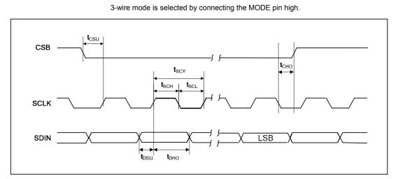
Figure 7 Control Interface Timing – 3-Wire Serial Control Mode (Write Cycle)
