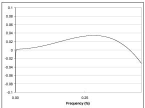
Figure 59 ADC Digital Filter Frequency Response
