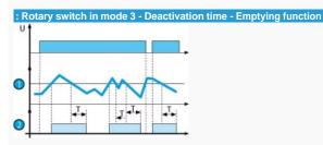
(level: 1 - off delay, function Dwn LS (Low Sensitivity:  $250~\Omega$  to  $5~k\Omega$ ) or Dwn St (Standard Sensitivity:  $5~k\Omega$  to  $100~k\Omega$ ) or Dwn HS (High Sensitivity:  $50~k\Omega$  to  $1~M\Omega$ ).
