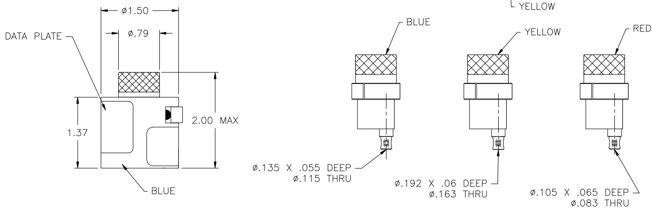
TYPICAL CONSTRUCTION DIAMETERS ARE MEASURED FROM TOP OF POSITIONER INSERTS
