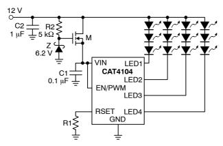
Figure 20. Single Supply Driving 12 LEDs
