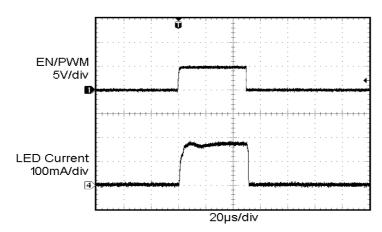
Figure 18. PWM 200 Hz, 1% Duty Cycle
