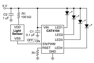
Figure 21. Daylight Detection
