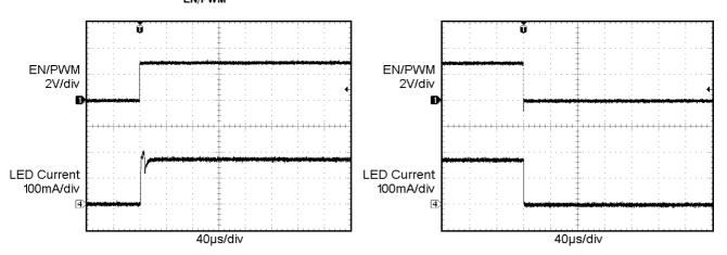
Figure 16. Power Up from Shutdown
