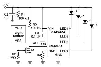
Figure 22. Nightlight Detection
