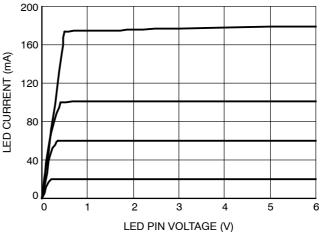
Figure 9. LED Current vs. RSET Resistor
