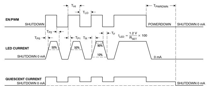
Figure 2. CAT4104 EN/PWM Timing
