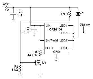
Figure 23. LED Current Derating
