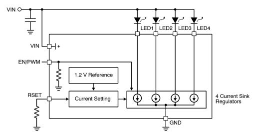
Figure 19. CAT4104 Functional Block Diagram
