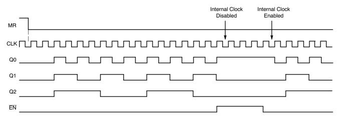
CASE 2: If the MR is de-asserted (H-L), after the Clock has transitioned low, the outputs will follow the third ensuing clock rising edge.
