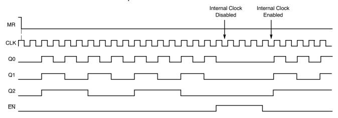
CASE 1: If the MR is de-asserted (H-L), while the Clock is still high, the outputs will follow the second ensuing clock rising edge.
