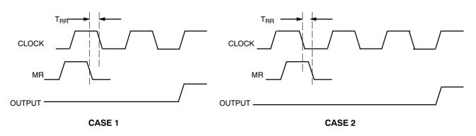
Figure 3. Reset Recovery Time
