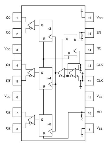
Warning: All  $\rm V_{CC}$  and  $\rm V_{EE}$  pins must be externally connected to Power Supply to guarantee proper operation.
