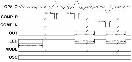
Figure 6. Timing Diagram for Single–Pulse Mode Detection
