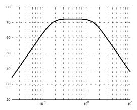
Figure 3. Plot Showing Typical Magnitude Response of Differential Amplifiers When Configured as a Bandpass Filter
