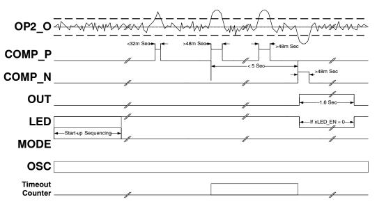
Figure 7. Timing Diagram for Dual–Pulse Mode Detection
