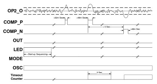
Figure 8. Timing Diagram for Two Pulses Outside Timeout Window
