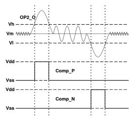
Figure 4. Plot Showing Functionality of Window Comparator for an Analog Input OP2\_O
