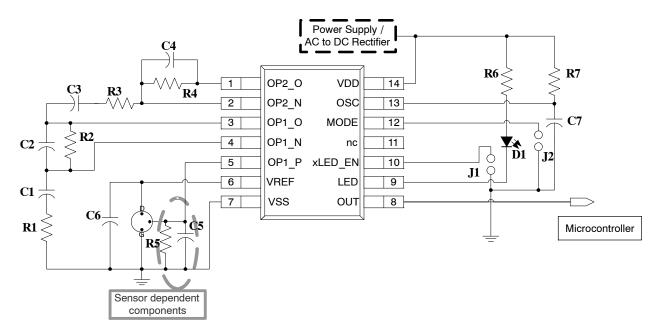
Figure 9. Typical Application Diagram Using NCS36000
