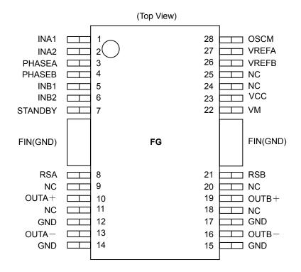
Please mount the FIN of the HSOP package to the GND area of the PCB.
