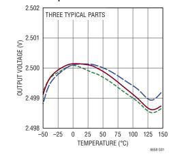
2.5V V<sub>OUT2</sub> Output Voltage Temperature Drift
