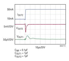
Figure 10. LT6658-2.5 Output 2 Response to 40mA Load Step
