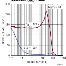
2.5V V<sub>OUT2</sub> Output Voltage Noise Spectrum I<sub>LOAD</sub> = 0mA
