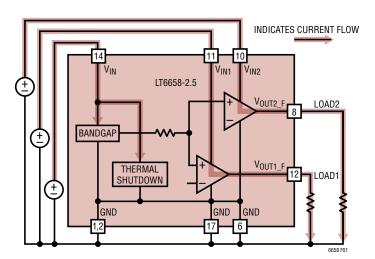
Figure 1. LT6658 Current Flow through the Supply Pins
