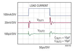
Figure 2. 10mA to 150mA Load Step on Vout1
