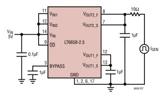
Figure 7. Load Current Response Time Test Circuit
