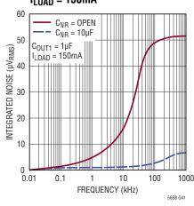
2.5V V<sub>OUT2</sub> Integrated Noise  $I_{LOAD} = 50 \text{mA}$
