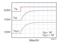
Figure 14. Start-up Response on the NR pin and  $V_{\mbox{\scriptsize OUT\_F}}$
