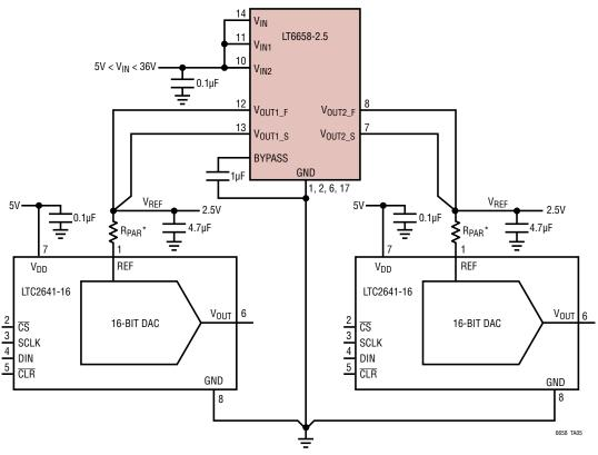
$^*$ R<sub>PAR</sub> is the parasitic resistance of the board trace and should be > 0.048 $\Omega$  to maintain good inl
