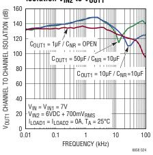
2.5V Channel to Channel Isolation  $V_{IN1}$  to  $V_{OUT2}$
