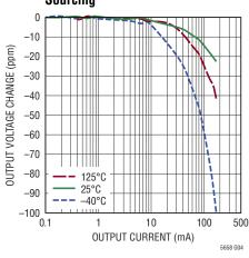
$2.5V\ V_{OUT2}\ Load\ Regulation,$ Sourcing
