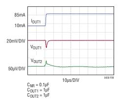
Figure 8. LT6658-2.5 Output 1 Response to 75mA Load Step
