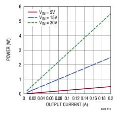
Figure 19. Power Dissipation vs Output Current
