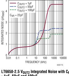
Figure 16. LT6658-2.5  $V_{OUT2}$  Integrated Noise with  $C_{NR}$  = 22 $\mu F$ and  $C_{0UT2} = 1\mu F$ ,  $50\mu F$  and  $100\mu F$
