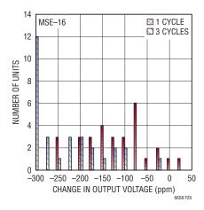
Figure 25. ΔV<sub>OUT1</sub> Due to IR Reflow Shift
