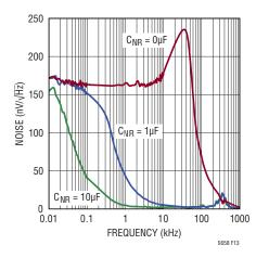
Figure 13. LT6658 Bandgap Output Voltage Noise
