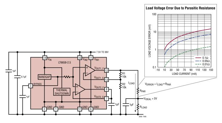
KELVIN SENSE ERROR:  $R_{PAR}$  WILL CAUSE AN ERROR  $V_{ERROR} = I_{LOAD} \bullet R_{PAR}$ . CONNECT THE TOP OF R1 DIRECTLY TO THE TOP OF  $R_{LOAD}$ . RESISTOR TOLERANCE ERROR: GAIN NETWORK ERROR CAN BE REDUCED BY USING A MATCHED RESISTOR NETWORK SUCH AS THE LT5400.
