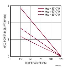
Figure 18. MSE Derating Curve
