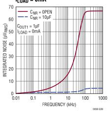
2.5V V<sub>OUT2</sub> Integrated Noise  $I_{LOAD} = OmA$
