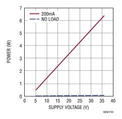
Figure 20. Power Dissipation vs Supply Voltage
