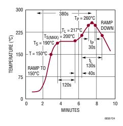
Figure 24. Lead Free Reflow Profile
