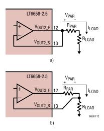
Figure 12. How to Make a Proper Kelvin Sense Connection
