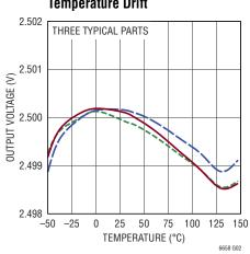
2.5V  $\mbox{V}_{\mbox{OUT1}}$  and  $\mbox{V}_{\mbox{OUT2}}$  Output Voltage vs Temperature with
