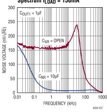
2.5V VOUT2 Output Voltage Noise Spectrum I<sub>I OAD</sub> = 50mA
