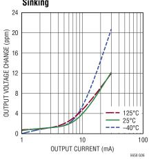
2.5V V<sub>OUT2</sub> Load Regulation, Sinking
