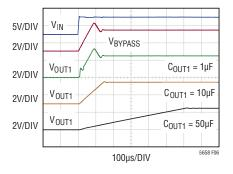
Figure 6. Start-Up Response on the BYPASS and V<sub>OUT1 F</sub> Pins
