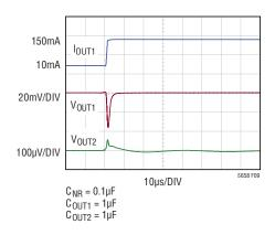
Figure 9. LT6658-2.5 Output 1 Response to 140mA Load Step
