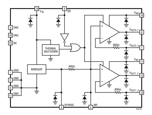
The LT6658 combines the low noise and accuracy of a high performance reference and the high current drive of a regulator. The LT6658 is a high performance regulator providing two precise low noise outputs with Kelvin sense pins. The isolated outputs maintain their precision even when large voltage or current transients exist on the adjacent channel.
