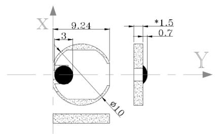
Mounting: The antenna is mounted with double sided adhesive tape that is attached to the antenna.
