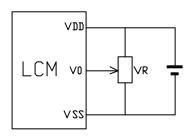
V<sub>DD~</sub>V<sub>0</sub>: LCD Driving voltage VR: 10k~20k
