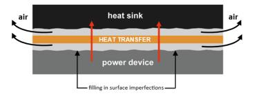
Note: during initial phase-change, it is recommended to re-check your torque settings if device utilizes a screw mounting system. Applying additional torque during initial phase change will thin the material bond line slightly leading to improved thermal performance.
