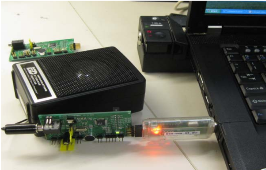
Figure 5 – A complete evaluation environment for ISD15100 device
